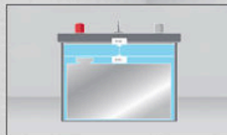
New design with deeper-set electrodes for greater acid capacity.
